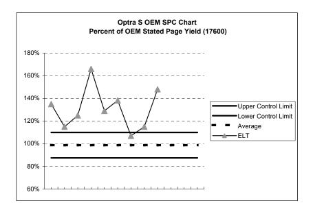
The Cartridge Toner Transfer Charts illustrate the efficiency of the cartridge. The compatibility of the toner and the charging components within the cartridge is critical to function. It is common for remanufactures to add more toner to the cartridge to compensate for inefficient toner transfer. The toner particle size distribution and OPC charging characteristics should be matches for optimum transfer efficiency.
